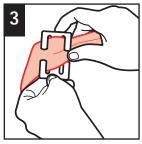
Thread both portions of the vehicle belt onto the locking clip.
